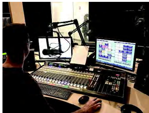
WFPK Studio 1 with Wheatstone LX-24 and VX drop-in and ENCO DAD.
